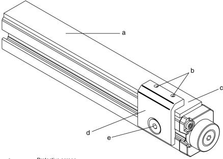
a = Protective screen b = Grub screw, M4x8
