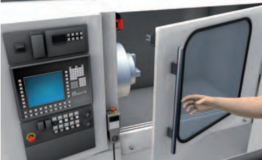
Safety Locking Device on a metal processing center with stopping times
