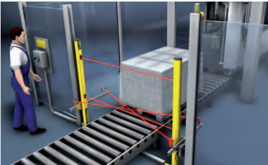
The Muting functionality enables pallets to pass by the active opto-electronic protective device without any process interruption with both the ASM1E and the ASM2E Safety Monitor.
